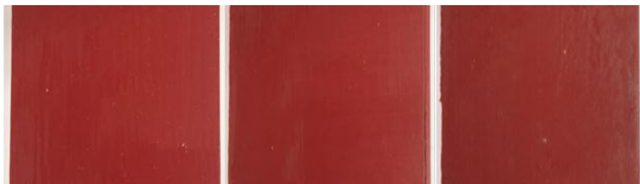
Figure 2: Coated PVC prototypes (10 x10 cm) with silicone based formulations, from left to right: 0 wt.% biocides (reference), containing 0.57 wt% and 2.57 wt. % of immobilised Econea-NCO.
