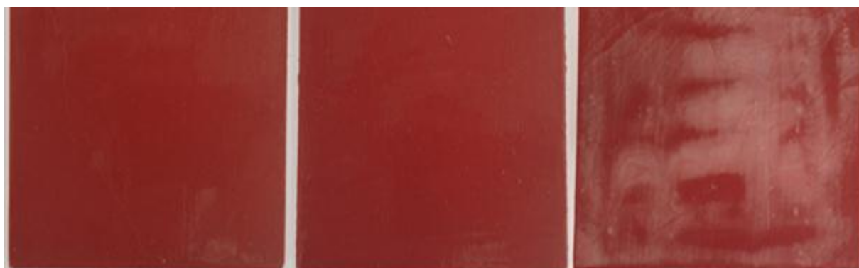
Figure 3: Coated PVC prototypes (10 x10 cm) with silicone based formulations, containing from left to right: 0.57 wt.%, 2.57 wt% and 5.0 wt.% of immobilised Irgarol.
