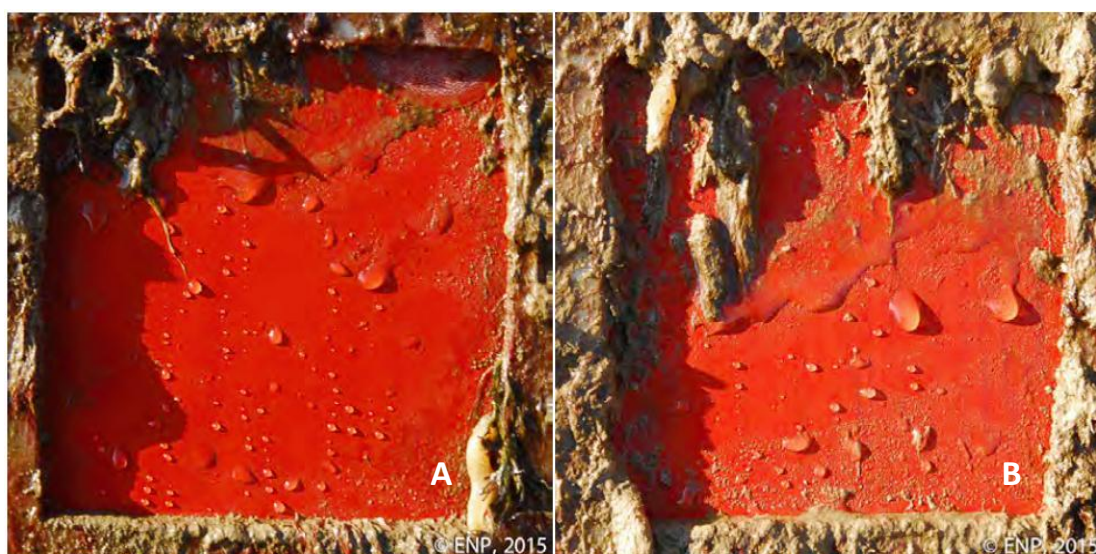
Figure 5: Coated PVC prototypes (10 x10 cm) with silicone based formulations, containing combined immobilised biocides: (A) 1.63 wt.% of immobilised Econea-NCO + Irgarol-NCO; and (B) the reference coating without biocides.
