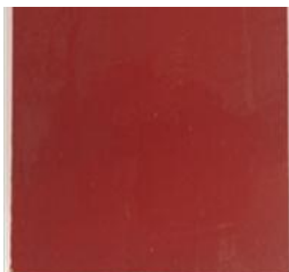
Figure 4: Coated PVC prototypes (10 x10 cm) with silicone based formulations, containing combined functional biocides: 1.53 wt.% of immobilised Econea + Irgarol.
