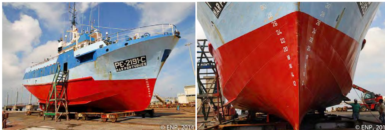
Figure 6. Vessel “Mar Português” painted with a new silicone based non-leaching coating. Photos gently provided by ENP, SA.
